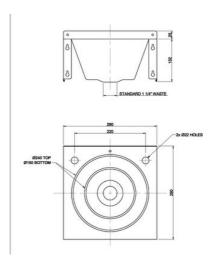
Washbasin top manufactured from 0.9mm thick, grade 1.4301 (304) stainless steel - high polish finish. The apron support is made from 0.9mm (430) material - high polish finish. Prepared for 32mm waste outlet and is supplied with two tapholes in the rear ledge. Note: It is not possible to fit an overflow in the bowl. Wall mounting by using the fixing holes provided in both the rear upstand and the rear apron fixing brackets. Screws and plugs are not supplied.
